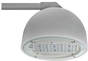
Copenhagen2 Large - LED module 8000 lm - LED - Power supply unit with DynaDimmer and constant light output (integrated) - Distribution medium 50 - Flat glass - - - - Side-entry for diameter 48 mm
