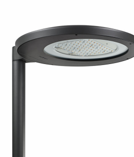
CitySoul gen2 Large - LED module 12000 lm - 830 warm white - Power supply unit with DALI and SystemReady interface - Safety class II - Distribution medium 50 - Clear glass - Gray - Philips standard surge protection level - - - Side-entry for diameter 60 mm
