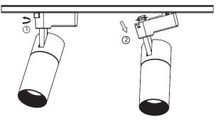
and standing for 15 minutes, the lamp holder can be directly Rotate the track head clip to the other end of the clip point and tilt the lamp holder can be directly the lamp according to the drawing until the track is pulled out.
