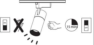
please do not contact the lamp cap directly with your hand to adjust when the light is lit.
