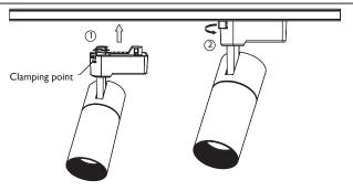
Put the track joint into the track, and rotate the track head clip past the clamping point to ensure that the conductor is in full contact.
