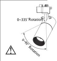
Only adjust the lighting angle when the power is off.
