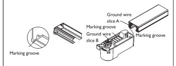
When installing, please first match the marking slot on the track joint to the marking slot on the track strip, and do not reverse install.
