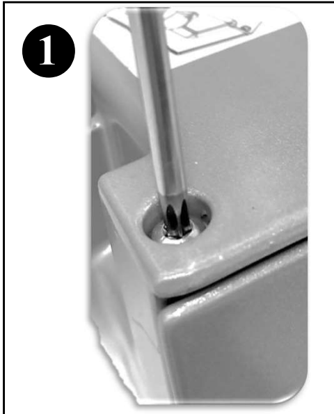
Unscrew the 4 screws of the driver housing
