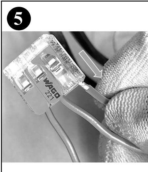
5 Disconnect the ground wire of the driver housing from the WAGO connector
