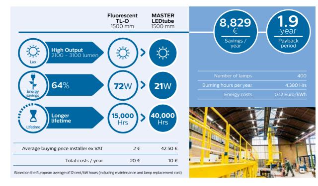
> Choose High Output LEDtubes for high light output with the best lm/w
